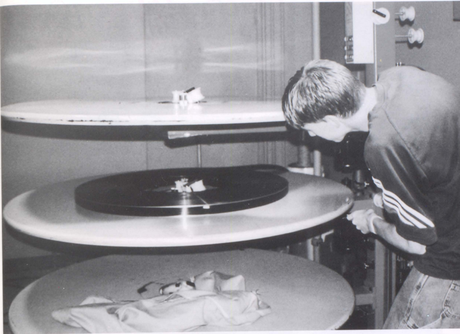
Senior Everett Shepherd threads film at Westglen 18 movie theater. " Depending on the movie, a one and a half hour movie will have five reels and a two and a half hour movie will have approximately eight to ten reels. I like being upstairs by myself where I don't have to worry about anything," Shepherd said.
